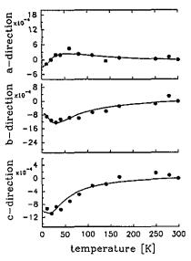
Figure 3. Experimentally determined differences of the normalized lattice parameters of  $NdCu_2$  and  $YCu_2$  (symbols). The lines represent the calculated results.
